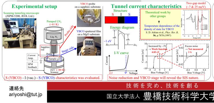
We proposed, fabricated, and evaluated a YBCO probe for realizing SIS junctions.
